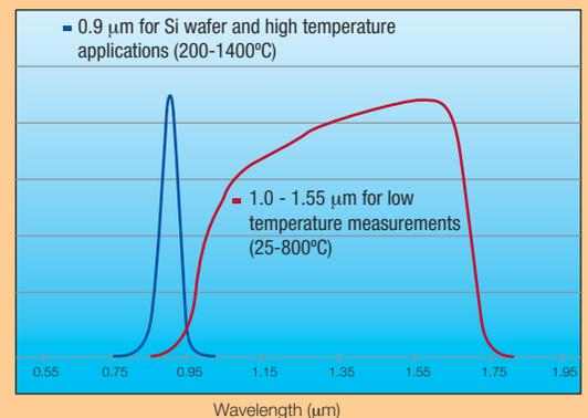
Detector wavelengths selected based on needs of application.
