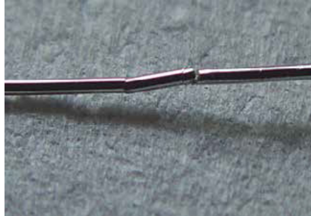
Image 14 - Crystallographic planes slippage
