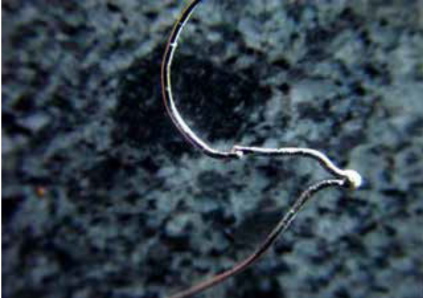
Image 13 - Grain size is 3-4 times bigger than the diameter of the wire
