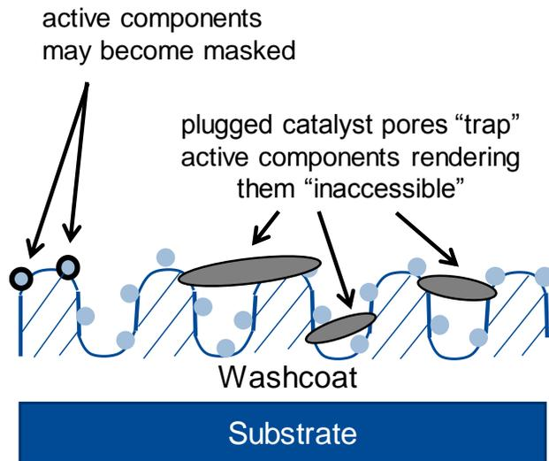
Figure 3. Schematic of catalyst in “as received” state
