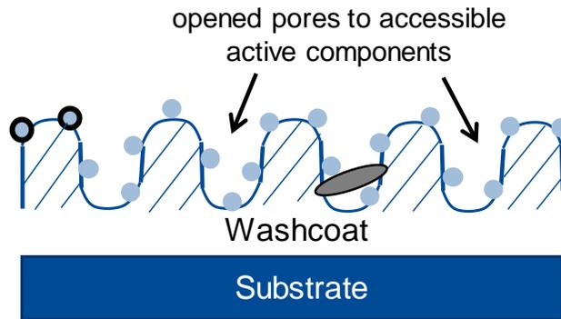
Figure 4. Schematic of catalyst restored by washing
