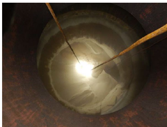
Figure 3. Donut-ring formation from molecular sieve caking in the dehydration vessel.
