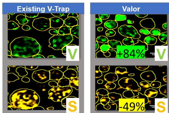
Testing results demonstrating greater activity retention of FCC catalyst using Valor<sup>®</sup>.
