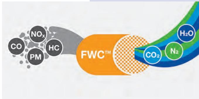
The Four-Way Conversion catalyst (FWC™) not only converts carbon monoxide, non-combusted hydrocarbons and nitrogen oxides into water, nitrogen and carbon dioxide, but also removes harmful particulate matter from the engine exhaust in gasoline-powered vehicles.
