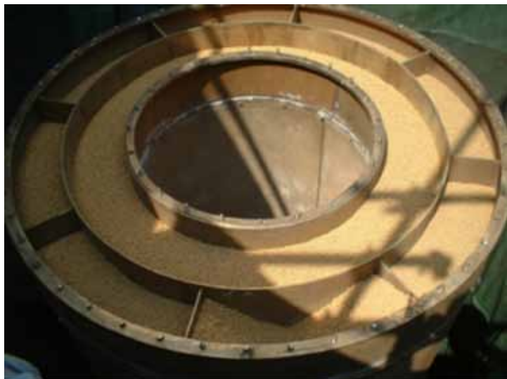
Figure 8: BASF state-of-the-art design ARF reactor
